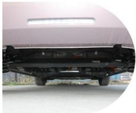
In terms of suspension, a combination of front MacPherson independent suspension and rear multi link independent suspension is adopted. Based on our previous test drive of the MINI EV Intelligent Electric iDD, we adopted sporty t uning style, bringing solid and agile driving pe rformance. At the same time, the chassis is equipped with power batteries and necessary battery brackets in the middle, so the entire chassis brings a stable and compact driving feel.
