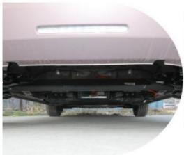
In terms of suspension, a combination of front MacPherson independent suspension and rear multi link independent suspension is adopted. Based on our previous test drive of the MINI EV Intelligent Electric iDD, we adopted sporty t uning style, bringing solid and agile driving pe rformance. At the same time, the chassis is equipped with power batteries and necessary battery brackets in the middle, so the entire chassis brings a stable and compact driving feel.
