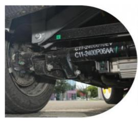
In terms of suspension, a combination of front MacPherson independent suspension and rear multi link independent suspension is adopted. Based on our previous test drive of the QQ ice cream Intelligent Electric iDD, we adopted sp orty tuning style, bringing solid and agile driv ing performance. At the same time, the chassis is equipped with power batteries and necess ary battery brackets in the middle, so the entire chassis brings a stable and compact driving feel.
