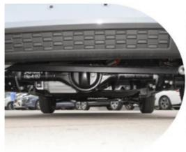
In terms of suspension, a combination of front MacPherson independent suspension and rear multi link independent suspension is adopted. Based on our previous test drive of the Chang an UNI-V Intelligent Electric iDD, we adopted a sporty tuning style, bringing solid and agile driving performance. At the same time, the chassis is equipped with power batteries and necessary battery brackets in the middle, so the entire chassis brings a stable and compact driving feel.
