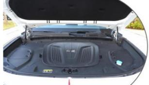
In terms of power, it is equipped with a Blue Whale 1.5T hybrid dedicated turb ocharged engine, with a maximum hor sepower of 170Ps and a maximum tor que of 260N  $\cdot$  m. With the assistance of an electric motor, the system's com prehensive maximum torque reaches 590N  $\cdot$  m. It is matched with a 6-spe ed three clutch electric drive transmis sion, which takes only 6.5 seconds to break 0-100km/h.
