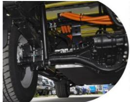
In terms of suspension, a combination of front MacPherson independent suspension and rear multi link independent suspension is adopted. Based on our previous test drive of the General EV pickup Intelligent Electric iDD, we adopted a sporty tuning style, bringing solid and agile driving performance. At the same time, the ch assis is equipped with power batteries and ne cessary battery brackets in the middle, so the entire chassis brings a stable and compact dri ving feel.
