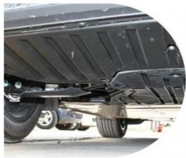
In terms of suspension, a combination of front MacPherson independent suspension and rear multi link independent suspension is adopted. Based on our previous test drive of the ID.4 CROZZ Intelligent Electric iDD, we adopted a sporty tuning style, bringing solid and agile driving performance. At the same time, the ch assis is equipped with power batteries and ne cessary battery brackets in the middle, so the entire chassis brings a stable and compact driving feel.
