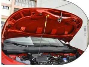
In terms of power, it is equipped with a Blue Whale dedicated turbocharged e ngine, with a maximum horsepower of 170Ps and a maximum torque of 260N • m. With the assistance of an electric motor, the system's comprehensive m aximum torque reaches 590N • m. It i s matched with a 6-speed three clutch electric drive transmission, which take s only 6.5 seconds to break 0-100km/h.
