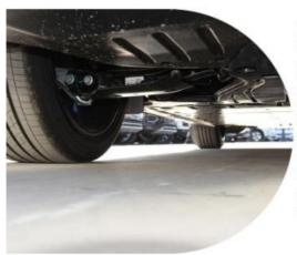
In terms of suspension, a combination of front MacPherson independent suspension and rear multi link independent suspension is adopted. Based on our previous test drive of the Chang an UNI-V Intelligent Electric iDD, we adopted a sporty tuning style, bringing solid and agile driving performance. At the same time, the chassis is equipped with power batteries and necessary battery brackets in the middle, so the entire chassis brings a stable and compact driving feel.
