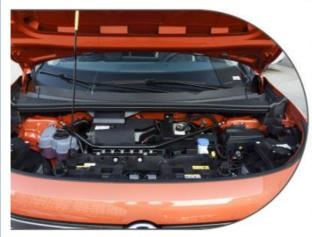
In terms of power, it is equipped with a Blue Whale 1.5T hybrid dedicated turb ocharged engine, with a maximum hor sepower of 170Ps and a maximum tor que of 260N • m. With the assistance of an electric motor, the system's com prehensive maximum torque reaches 590N • m. It is matched with a 6-spe ed three clutch electric drive transmis sion, which takes only 6.5 seconds to break 0-100km/h.
