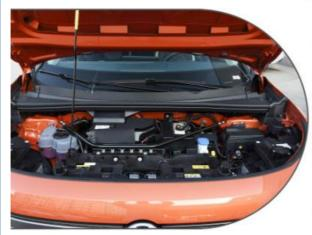
In terms of power, it is equipped with a Blue Whale 1.5T hybrid dedicated turb ocharged engine, with a maximum hor sepower of 170Ps and a maximum tor que of 260N • m. With the assistance of an electric motor, the system's com prehensive maximum torque reaches 590N • m. It is matched with a 6-spe ed three clutch electric drive transmis sion, which takes only 6.5 seconds to break 0-100km/h.
