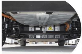
In terms of suspension, a combination of front MacPherson independent suspension and rear multi link independent suspension is adopted. Based on our previous test drive of the Auspic ious geometry Intelligent Electric iDD, we ado pted a sporty tuning style, bringing solid and agile driving performance. At the same time, the chassis is equipped with power batteries and necessary battery brackets in the middle, so the entire chassis brings a stable and compact driving feel.
