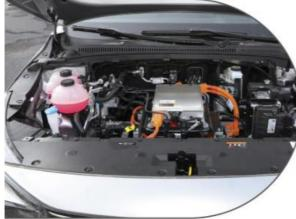
In terms of power, it is equipped with a Blue Whale dedicated turbocharged e ngine, with a maximum horsepower of 170Ps and a maximum torque of 260N • m. With the assistance of an electric motor, the system's comprehensive m aximum torque reaches 590N • m. It is matched with a 6-speed three clutch electric drive transmission, which takes only 6.5 seconds to break 0-100km/h.
