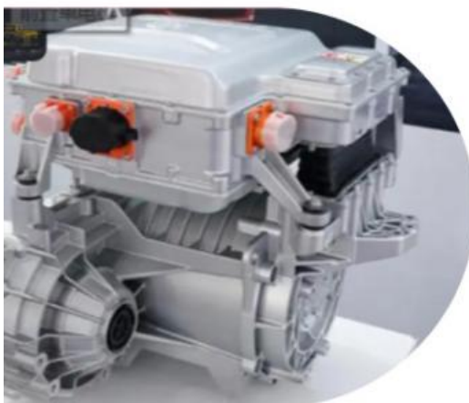
Motor type: permanent magnet synchronous - total power of motor (kW): 55- total torque of motor (Nm): 170, as shown in the diagram
