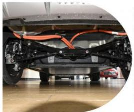
In terms of suspension, a combination of front MacPherson independent suspension and rear multi link independent suspension is adopted. Based on our previous test drive of the Song P LUS EV Intelligent Electric iDD, we adopted as porty tuning style, bringing solid and agile dri ving performance. At the same time, the chas sis is equipped with power batteries and nece ssary battery brackets in the middle, so the en tire chassis brings a stable and compact driving feel.
