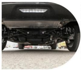
In terms of suspension, a combination of front MacPherson independent suspension and rear multi link independent suspension is adopted. Based on our previous test drive of the Song P LUS DM-I Intelligent Electric iDD, we adopted a sporty tuning style, bringing solid and agile driving performance. At the same time, the chassis is equipped with power batteries and necessary battery brackets in the middle, so the entire chassis brings a stable and compact driving feel.
