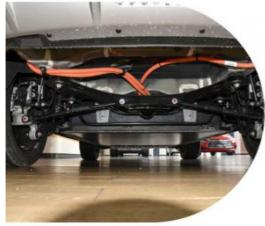
In terms of suspension, a combination of front MacPherson independent suspension and rear multi link independent suspension is adopted. Based on our previous test drive of the Song P LUS EV Intelligent Electric iDD, we adopted as porty tuning style, bringing solid and agile dri ving performance. At the same time, the chas
