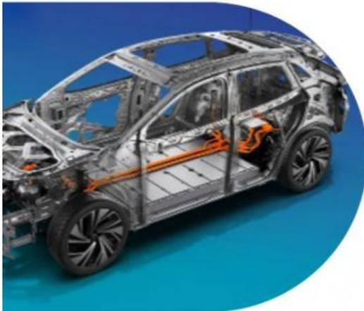
The diagram of over 29% hot formed steel plate \* is provided as a schematic diagram
