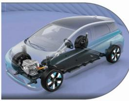
In terms of power and battery configuration, it is the focus of the BYD Dolphin 2023 Fashion Edition. The pure electric range announced by the Ministry of Industry and Information Technology is 420km, with a total power of 70kW and a total torque of 180N • m. In addition, it is equipped with BYD's latest Blade battery pack, which has further improved battery capacity and performance.
