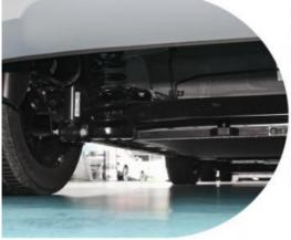
In terms of suspension, a combination of front MacPherson independent suspension and rear multi link independent suspension is adopted. Based on our previous test drive of the Haitun
