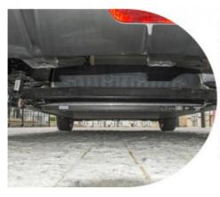
In terms of suspension, a combination of front MacPherson independent suspension and rear multi link independent suspension is adopted. Based on our previous test drive of the Chang an UNI-V Intelligent Electric iDD, we adopted a sporty tuning style, bringing solid and agile driving performance. At the same time, the chassis is equipped with power batteries and necessary battery brackets in the middle, so the entire chassis brings a stable and compact driving feel.
