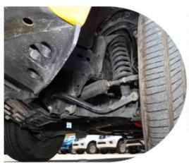
In terms of suspension, a combination of front MacPherson independent suspension and rear multi link independent suspension is adopted. Based on our previous test drive of the Pickup Car Intelligent Electric iDD, we adopted sport y tuning style, bringing solid and agile driving performance. At the same time, the chassis is equipped with power batteries and necessary battery brackets in the middle, so the entire ch assis brings a stable and compact driving feel.
