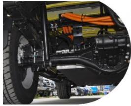
In terms of suspension, a combination of front MacPherson independent suspension and rear multi link independent suspension is adopted. Based on our previous test drive of the General EV pickup Intelligent Electric iDD, we adopted a sporty tuning style, bringing solid and agile driving performance. At the same time, the ch assis is equipped with power batteries and pe
